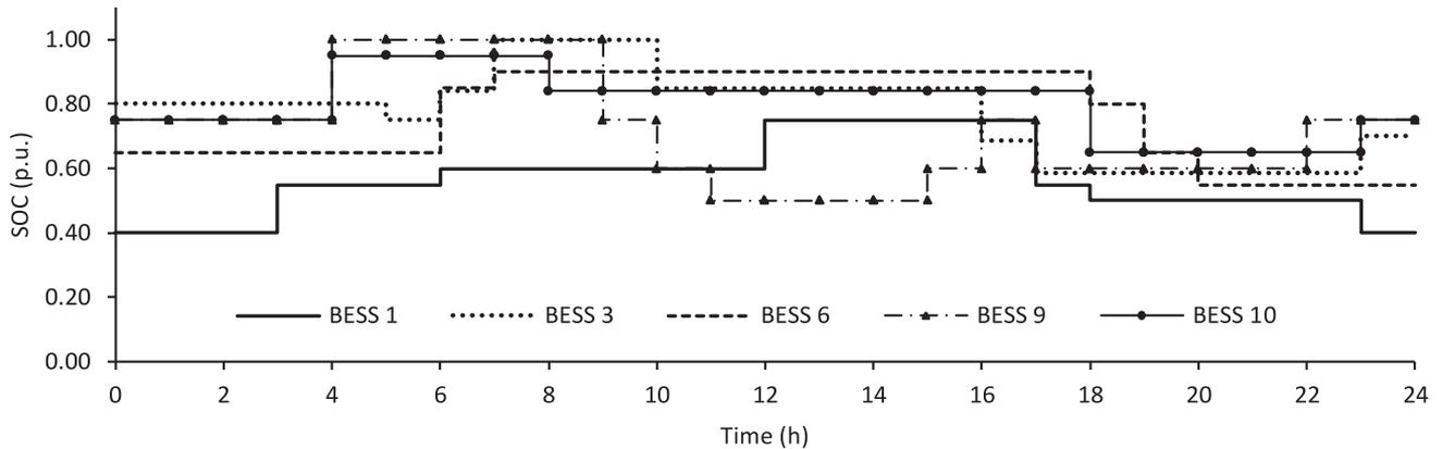
Fig. 10. SOC profiles of BESS after market dispatch in Case 3.
