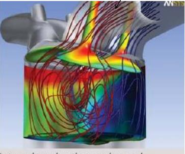
Internal combustion engine and the flow inside modeled using ANSYS FLUENT software
